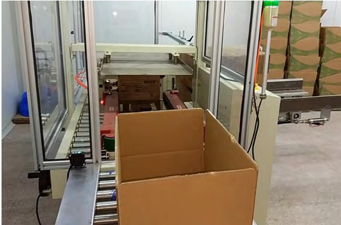
It is a vertical carton erector or case former. This machine erects flat-fold cartons and seals bottoms with tape as boxes.
