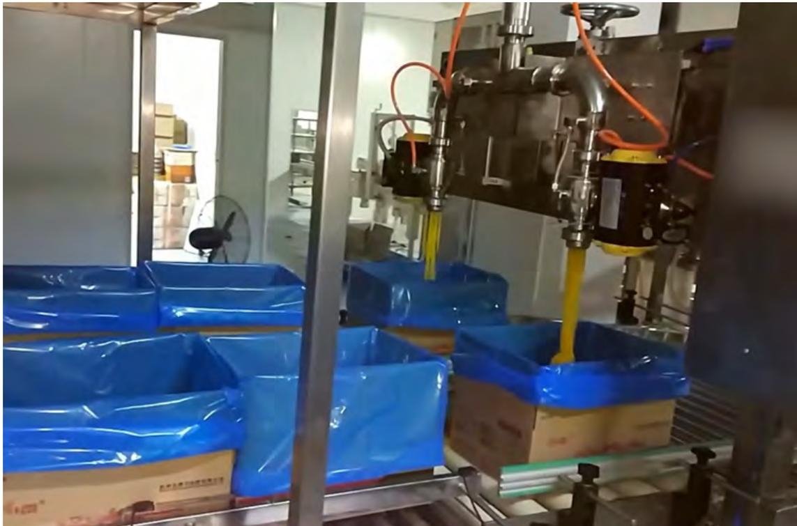
This is a double-head weigh filling machine. Grade 304 stainless steel frame and 316L stainless steel product-contact parts.
